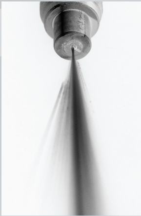
Fouled Injector Without Gen 49D
